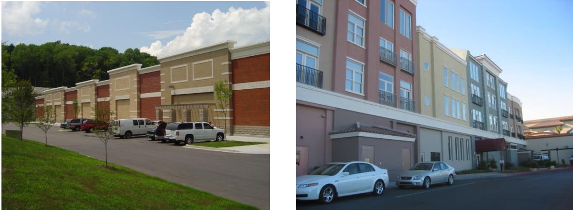
Figure 6-16: This figure shows two methods of using architectural features to create wall surface relief on wall elevations that are not the primary elevation.
